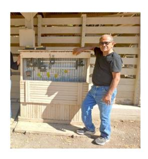
WEIGHTS AND MEASURES INSPECTORS CERTIFY DEVICES USED IN COMMERCE THAT WEIGH, MEASURE, OR COUNT A PRODUCT ARE ACCURATE AND WITHIN TOLERANCE ANNUALLY. UPON THE COMPLETION OF AN INSPECTION A SEAL, AS PICTURED ABOVE, IS PLACED ON THE DEVICE.
