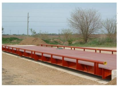
Pictured to the left is a vehicle scale. When loaded the county's weight truck weighs 38,000 pounds including sixteen 1000 lb blocks. With the truck certified at that weight, it is used to seal vehicle scales. The on-board crane makes quick work of loading and unloading blocks when certifying livestock, dormant, and platform scales.
