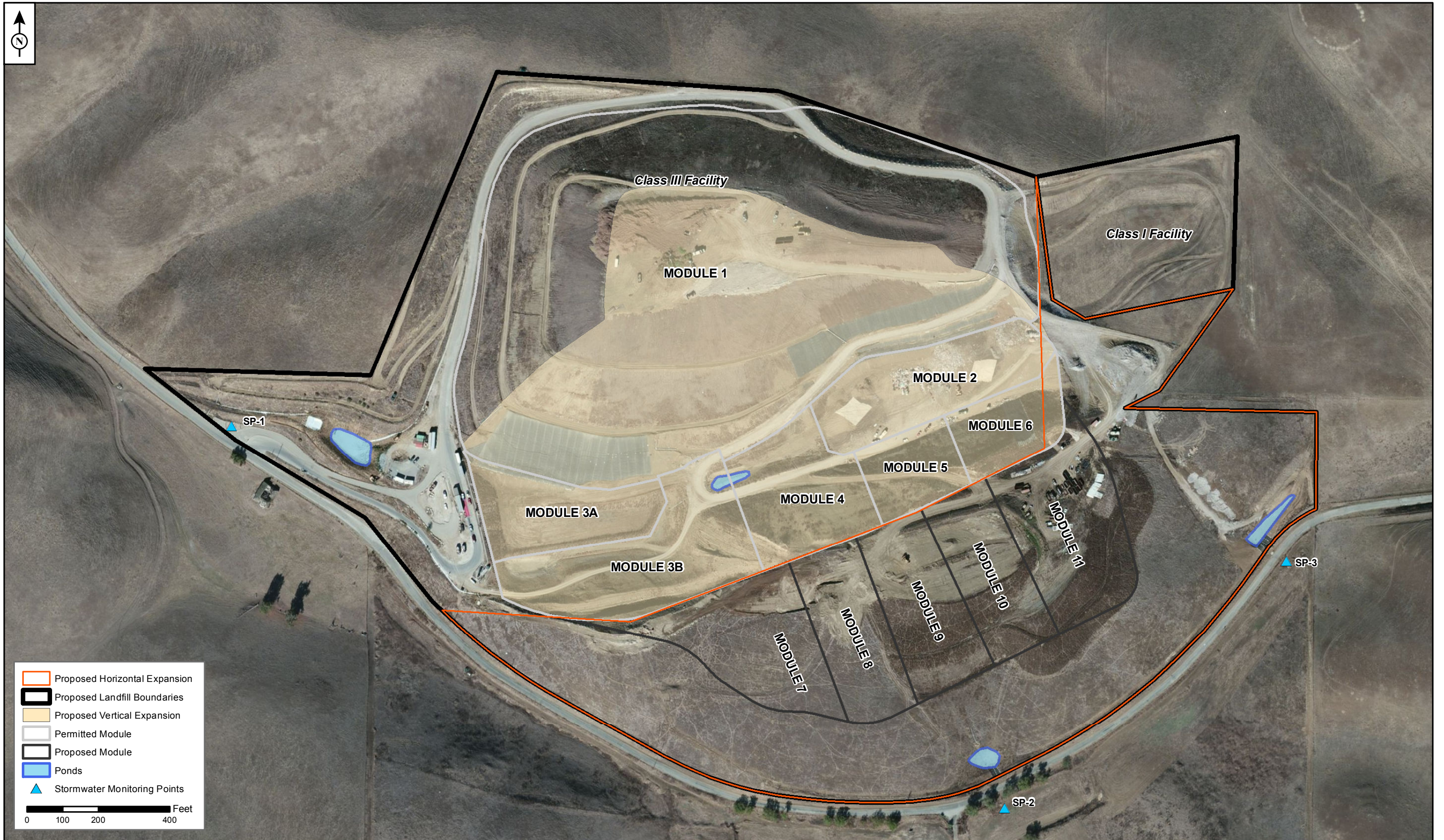
Figure 6. Stormwater Sampling Points and Ponds JOHN SMITH ROAD LANDFILL EXPANSION PROJECT
