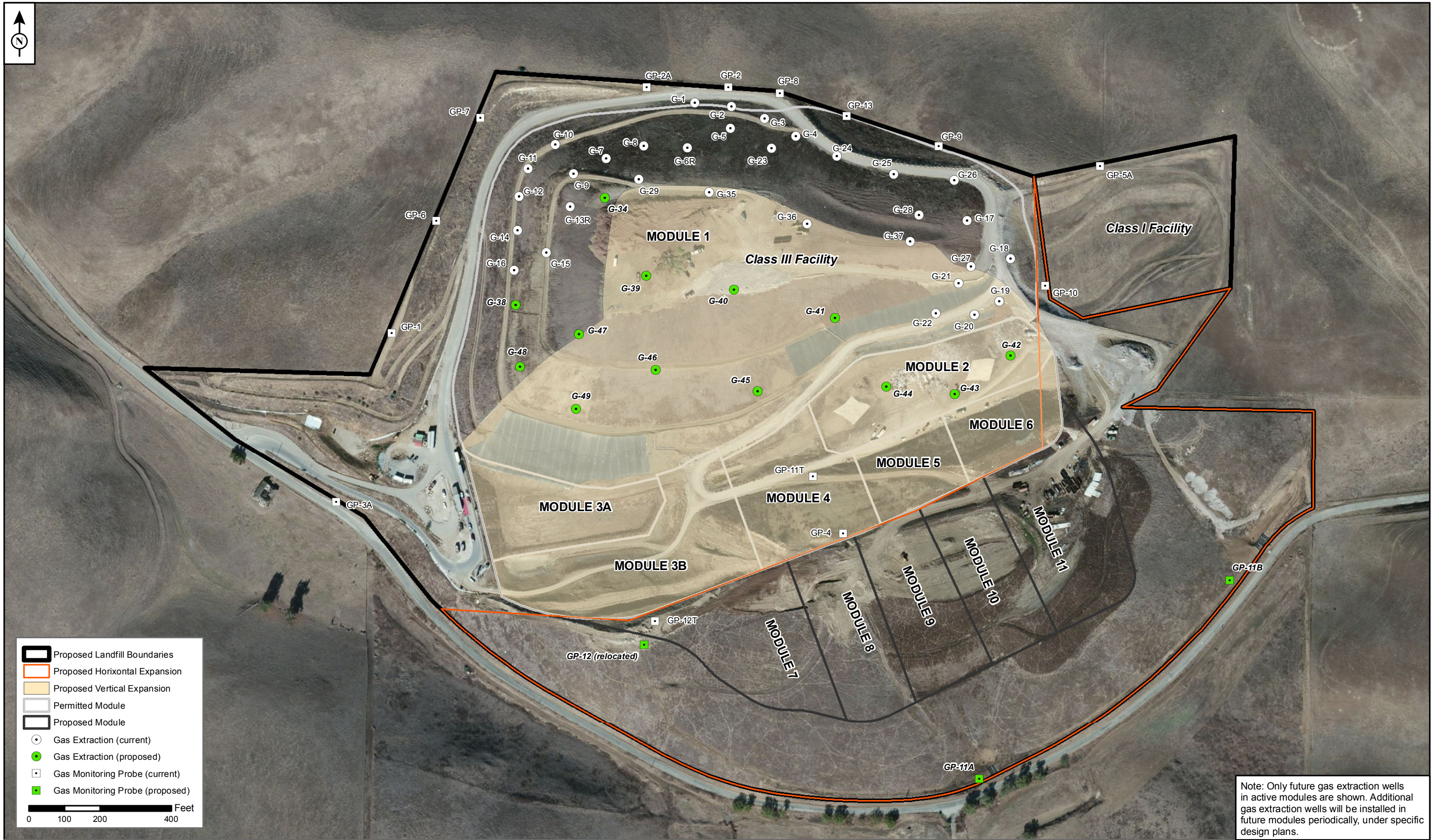
Figure 5. Landfill Gas Monitoring and Extraction Points JOHN SMITH ROAD LANDFILL EXPANSION PROJECT
